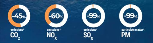
\*Estimated data comparing the emissions of the Nerea powered by LNG with those of a similarly sized ship powered by MDO
